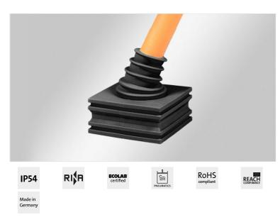
The KT-DPF grommets accept a wide range of cable diameters. A great benefit when the exact cable diameter is not known in advance. Due to the flexibility and unique pyramid shape, routing and flexible positioning of rigid cables is much easier compared to using conventional cable glands.
